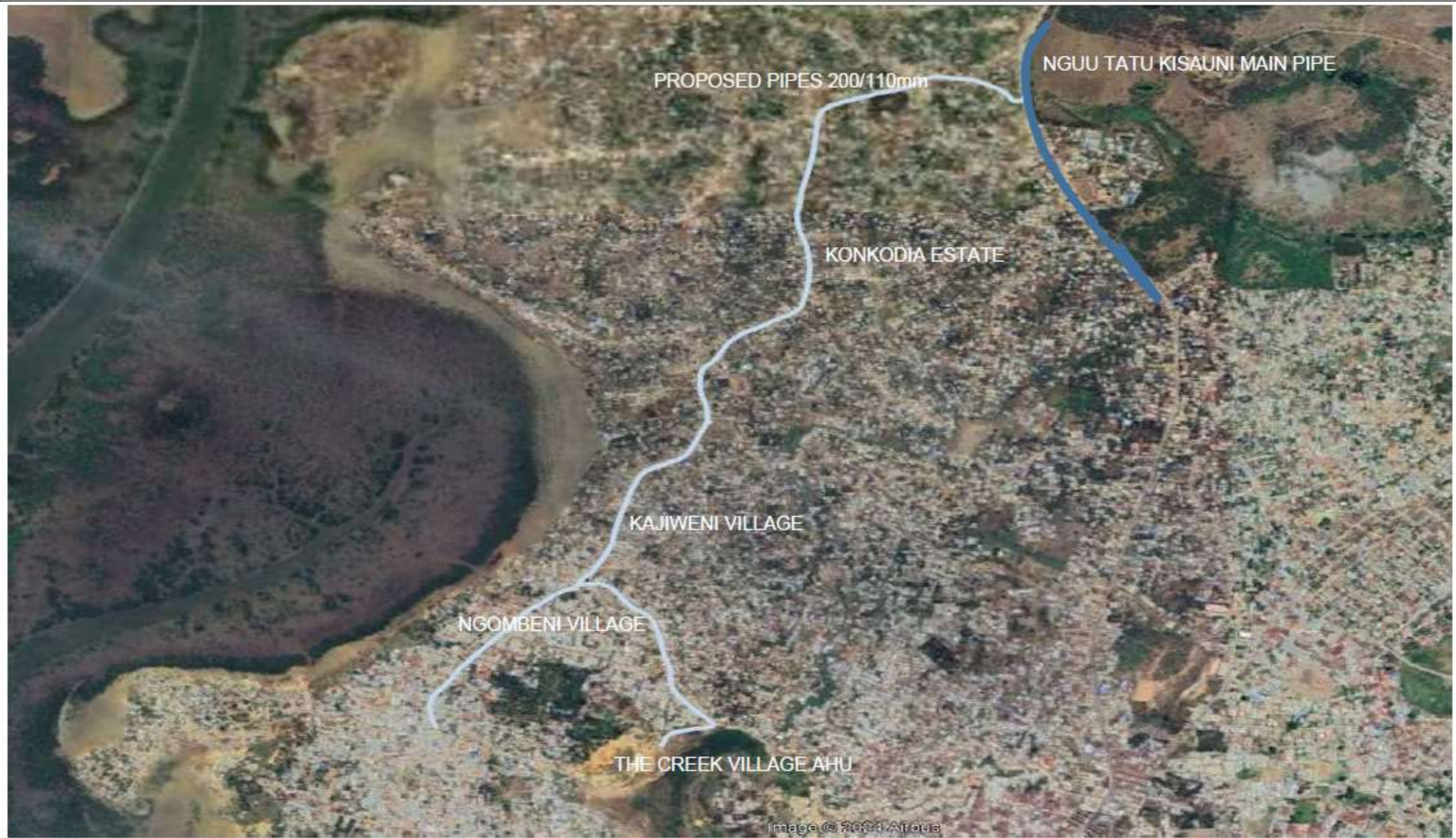
CWWDA /PIPE LAYOUT/02: SATELLITE IMAGE: WATER PIPELINE EXTENSIONS TO CREEK VILLAGE AHU.
